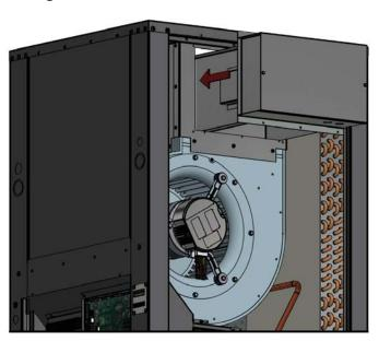
**3. Slide plenum heater** *UP* approximately 3/8". Top flange of heater is held in top groove of blower assembly and requires no fasteners. Install 3 screws through bottom flange of heater through pre-punched holes in heater and blower assembly.
