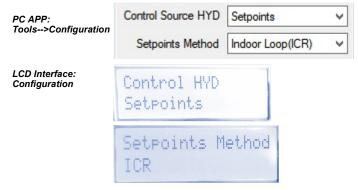
ICR (Internal Circulator Relay) is the default method and uses the **Indoor OUT** temperature probe inside the unit for temperature control. Its value is displayed in the **Tank Temperature** box on the PC App's **View-->Setpoint Control** window, shown below. If this temperature shows **NC**, then either the probe is not connected to the board or there is a problem with it.
