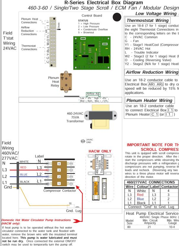
Low Voltage Wiring (24VAC)
