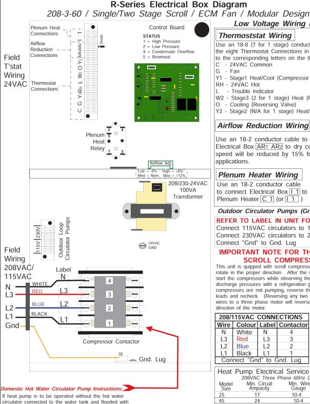
water, remove the brown wire with the insulated terminal located here. This pump is water lubricated and must not be run dry. Once connected the external ON/OFF switch may be used to temporarily turn the pump off.
