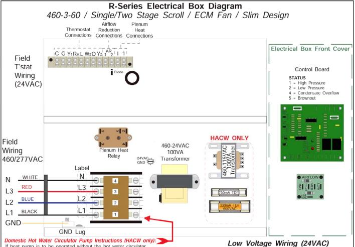
If heat pump is to be operated without the hot water circulator connected to the water tank and flooded with water, remove the brown wire with the insulated terminal located here. This pump is water lubricated and must not be run dry. Once connected the external ON/OFF switch may be used to temporarily turn the pump off.
