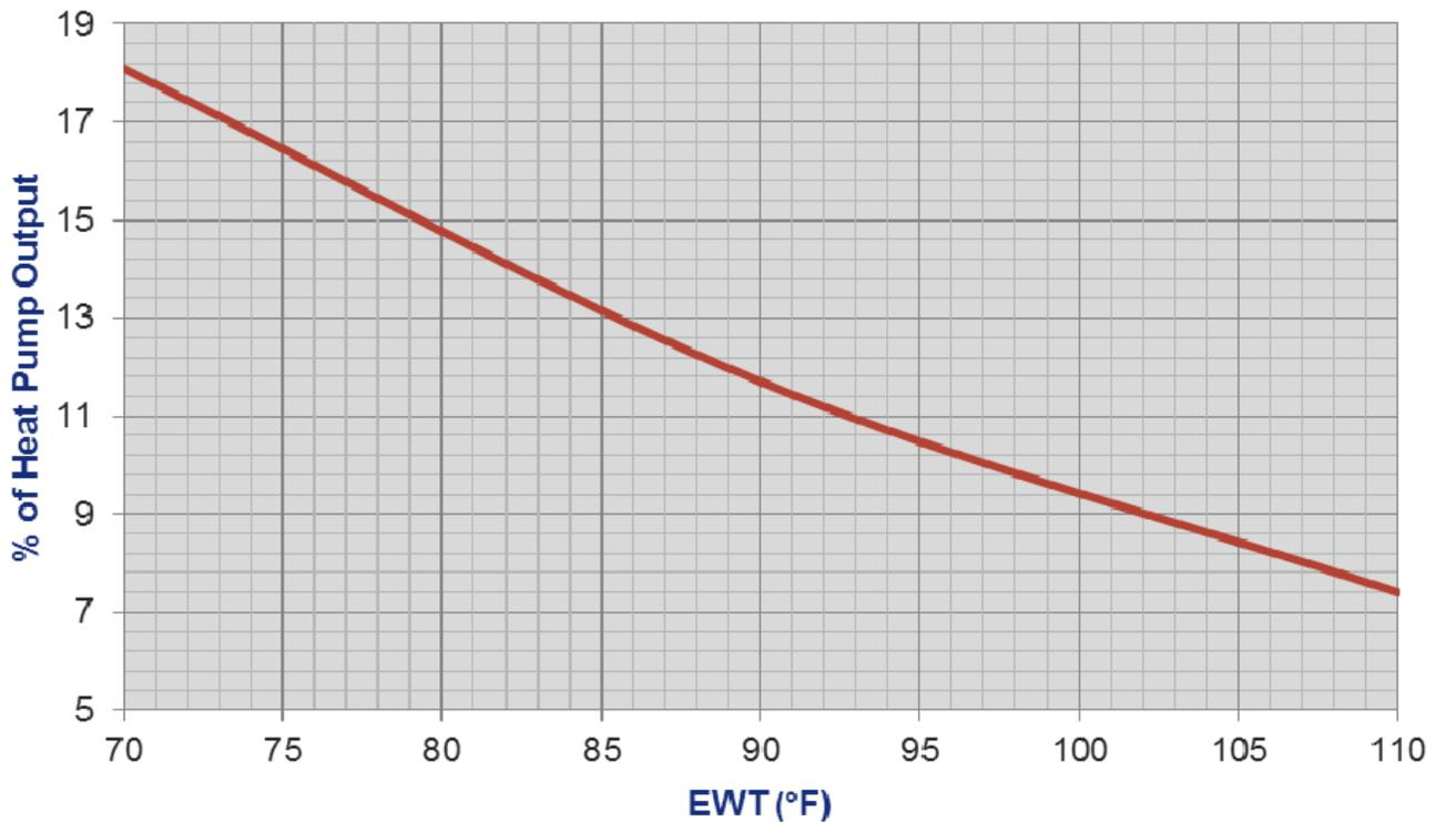
These charts are based on a Nordic IFM-48 used with a nominal 4 ton heat pump, in a typical heating mode condition of 25°F (-4°C) evaporating temperature and 105°F (41°C) condensing temperature, with a hydronic system water flow of 1.0 gpm.
