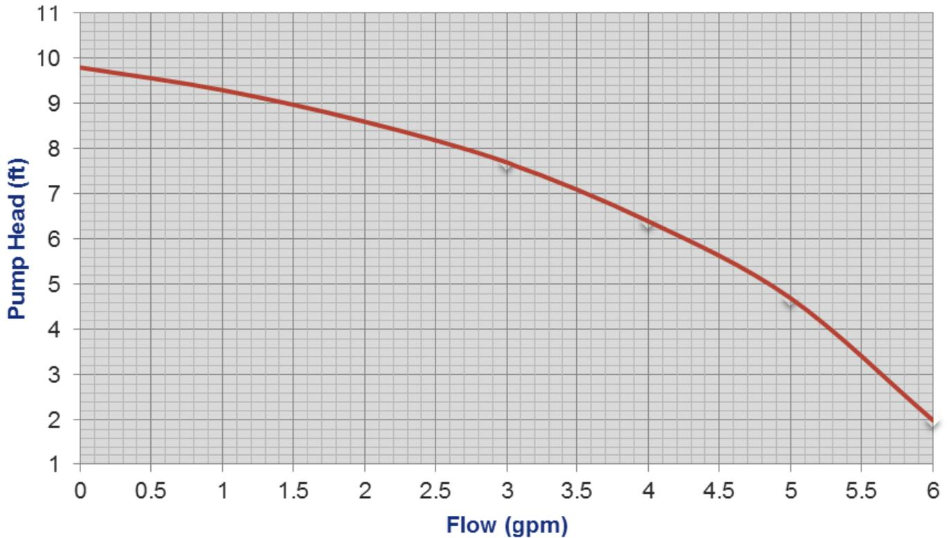
Factors contributing to the pump head include the pressure drop of the hydronic circuit connected to the IFM, and pressure drop through the IFM's internal heat exchanger. See following tables for total combined pressure drop information.
